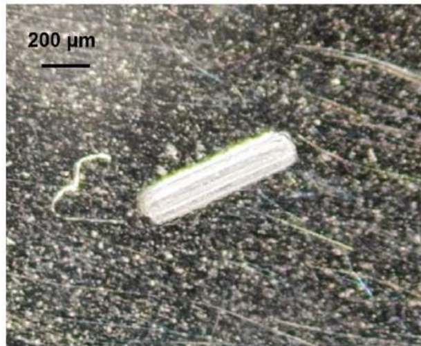
Figure S13. A cylinder with an inner diameter of approximately 100 μm and an outer diameter of approximately 200 μm.
