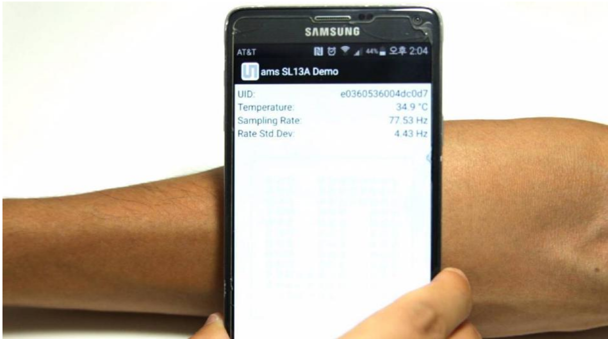
Movie s2. Movie of temperature sensing with a smart phone activated by the wireless NFC interface.
